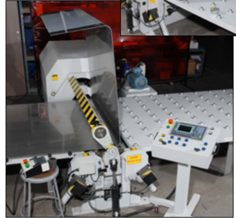
5 Axis C.N.C. Specialized Roll Forming System performs complex forming program to produce a 2" radius square tank in 2-ft / 6-ft squares.
