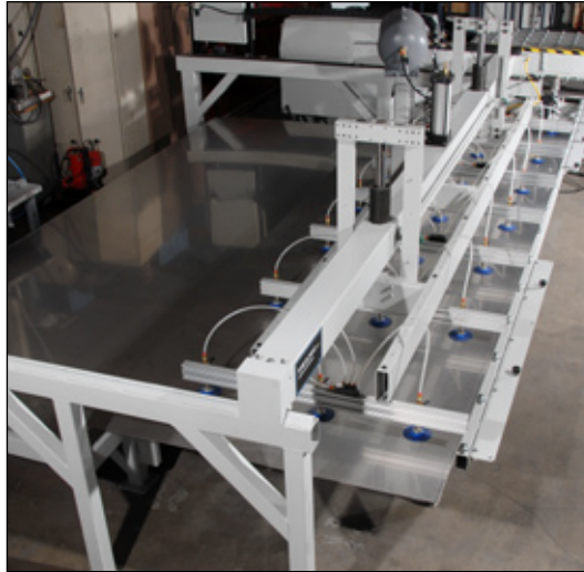
S.S. Sheet Metal De-Stacker vacuum lifts 3/16" sheets up to 144" length x 60" width and places on transfer table automatically.
