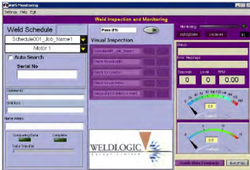
Developed with one of our major customers and proven in a production environment, AWS Monitor is a Windows based, real time data acquisition system, designed to run on a standard PC or laptop.
